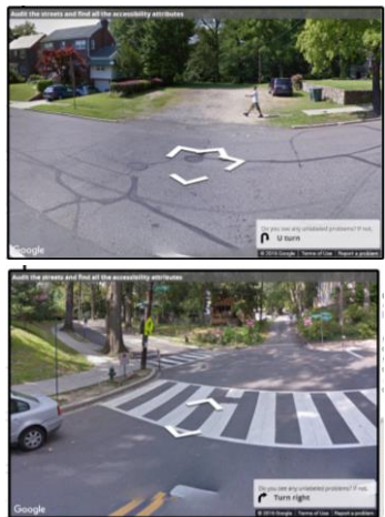
Fig. 2: Two example issues found in Project Sidewalk: (top) A pedestrian walking on grass after a sidewalk ends and (bottom) a newly painted crosswalk to an intersection without a curb ramp.
